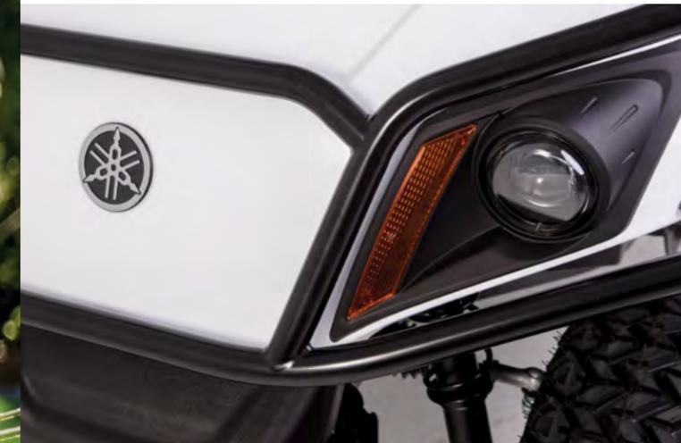
Yamaha Genuine front brush guard has a black powder-coated finish with 1¼" diameter tubing to fit a variety of mounts for additional lighting accessories.
