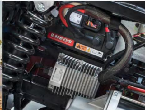
Toyota Industries-built motor controller unit.
